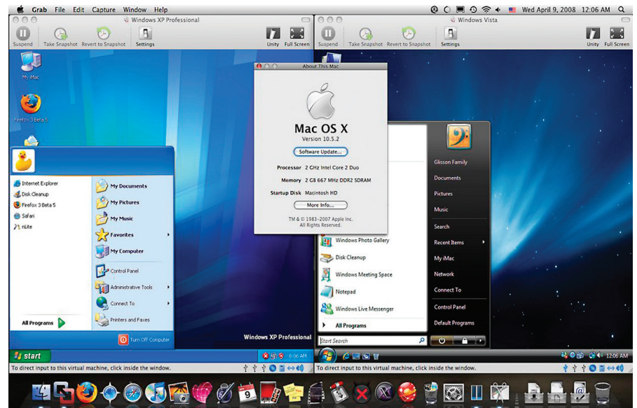
An iMac computer, with VMware Fusion, which enables it to run Windows XP Pro on the left screen, Windows Vista Home on the right, and Mac OS X Leopard in the background.
